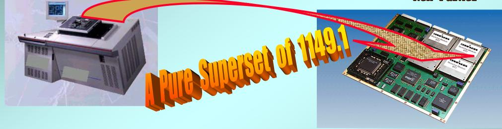
The first important characteristic to note about the IEEE 1149.4 Std is that it is intended for use with lower frequencies: from DC to around 10 MHz. If this seems like a serious limitation, consider the fact that virtually all the boards tested with ICT over the last 25 years have had their analog components tested at 10 kHz or less!
